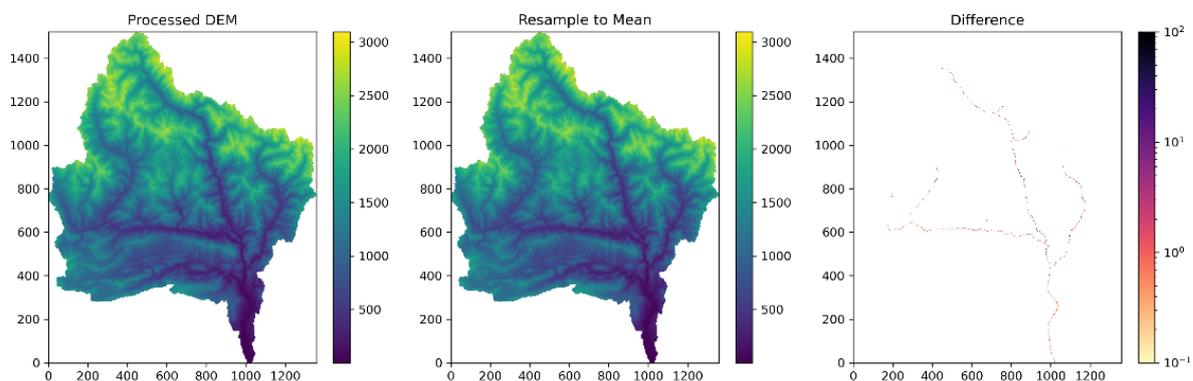
**Figure 1:** Comparison between the processed DEM and the input DEM resampled using the mean of the initial 25m resolution DEM. The difference between the two is plotted showing where the river network has been carved into the mean DEM.
