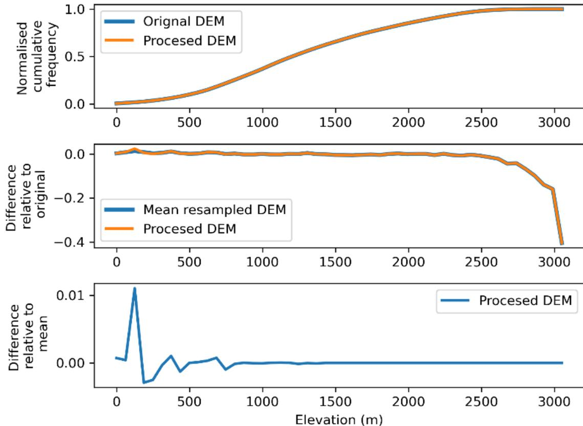
**Figure 2:** Cumulative distribution of elevation for the original 25 m DEM and the processed DEM. The difference in the distribution of the mean resampled DEM at 50 m resolution and the processed DEM is shown. It can be seen that both are similar, with an under-representation of high topography. The difference between the mean and processed DEM is shown. Here the impact of the carving can be seen, with an increase in low topographies for the processed DEM, where dams have been removed.
